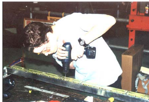
(d) High school student mounting detector circuits along a frictionless air track.
