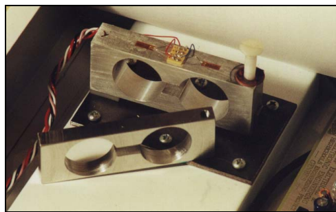
(d) Strain gauge bridge measures vertical displacement of the scale pan.
