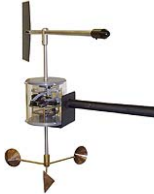
(a) Digital Anemometer – measures wind direction and wind speed
