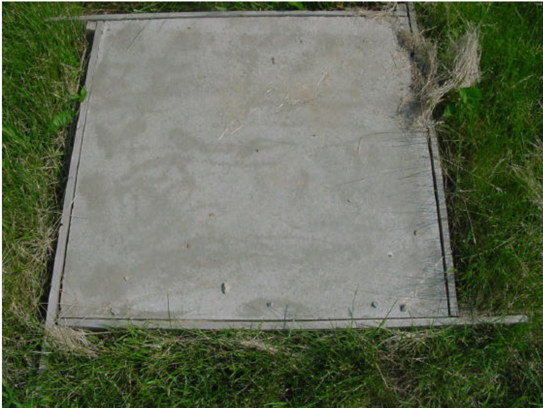
Figure 3: A silica fume concrete slab used in the pilot project
