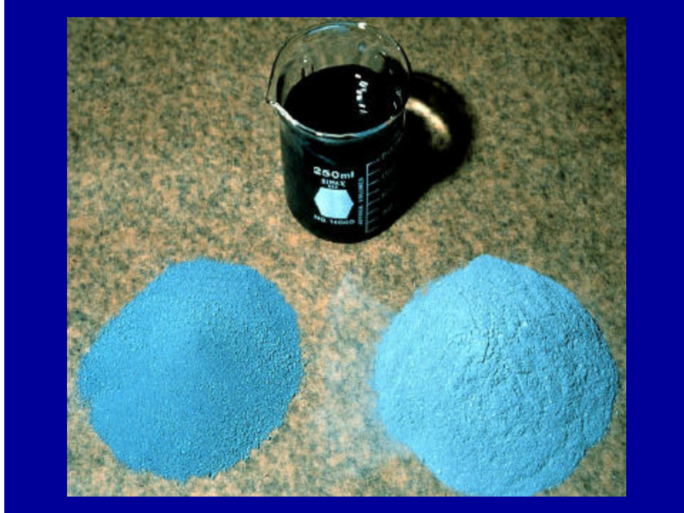
Figure 1: Various forms of silica fume Photo courtesy of the Silica Fume Association
