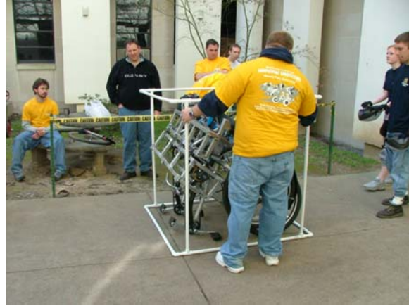
Figure 1: A Moonbuggy (left) is a human-powered vehicle that must fit or be collapsible to fit into a 4 foot cubic volume (right) and be carried 20 feet by its two drivers (1 male and 1 female).
