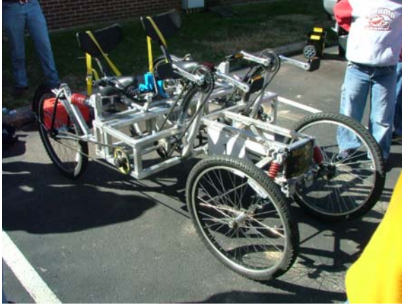
Figure 1: A Moonbuggy (left) is a human-powered vehicle that must fit or be collapsible to fit into a 4 foot cubic volume (right) and be carried 20 feet by its two drivers (1 male and 1 female).
