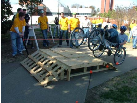
Figure 2: The course was 0.6 miles long and included obstacles made out of wood (left) and gravel (right) that simulated lunar terrain. The wooden obstacles were designed and constructed by freshman engineering physics students.
