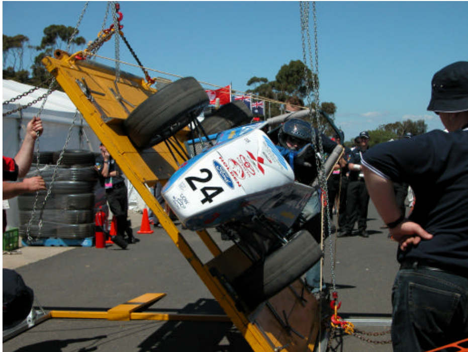
Photo 6 – 2004 Car, “Roger Ramjet” during the Tilt Test
